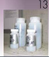
Fly ash comes from the small particles of incinerated waste that become airborne. The fly ash is captured in the baghouse and tested before finally being disposed in a landfill.
