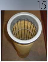
After lime and carbon are added, the flue gas is then passed through the fabric filter baghouse which captures acids, metals and particulate matter.
