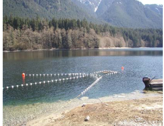
Above Left: Two rotary screw traps capture smolts on the Upper Capilano River. Above Right: Net traps capture smolts along the shoreline of Capilano Reservoir.
