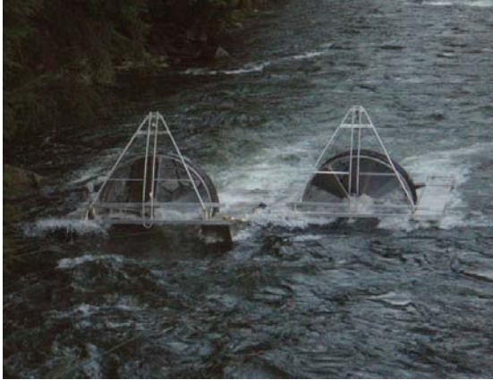
Above Left: Two rotary screw traps capture smolts on the Upper Capilano River. Above Right: Net traps capture smolts along the shoreline of Capilano Reservoir.
