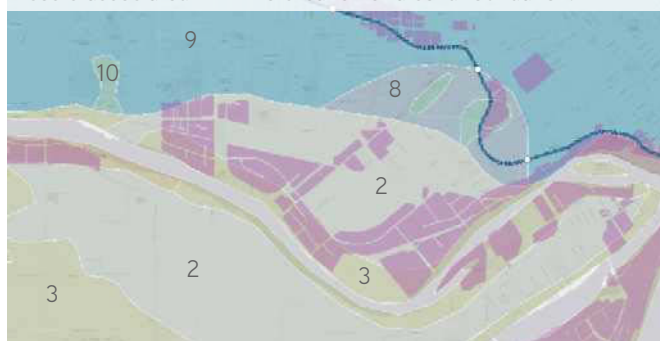
The peat (2) and silt/clay (3) of Big Bend result in significant costs associated with the creation of a solid foundation.
