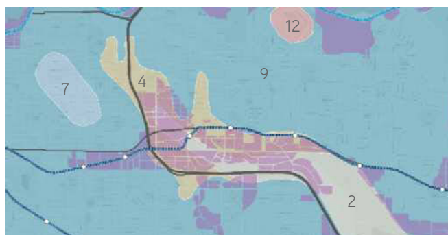
The peat (2) and sand/silt (4) of Still Creek, Burnaby may result in higher costs associated with earthquake stabilization.
