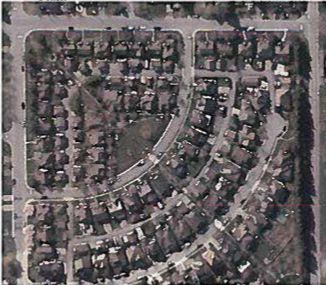
Figure 4.2 Illustrates a curvilinear block and street pattern with a modified H-shaped subdivision configuration
