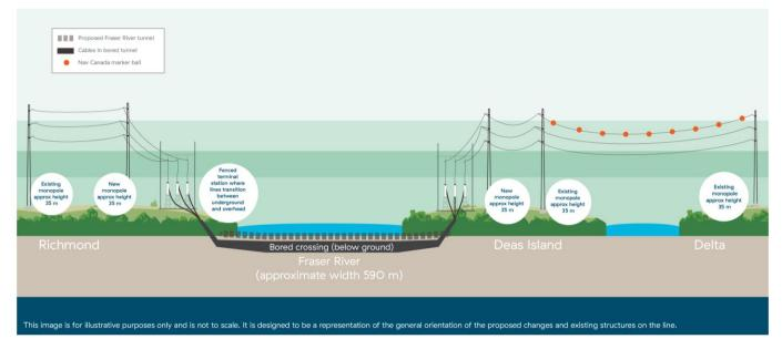
A new underground line separate from the Province's proposed immersed tube tunnel
