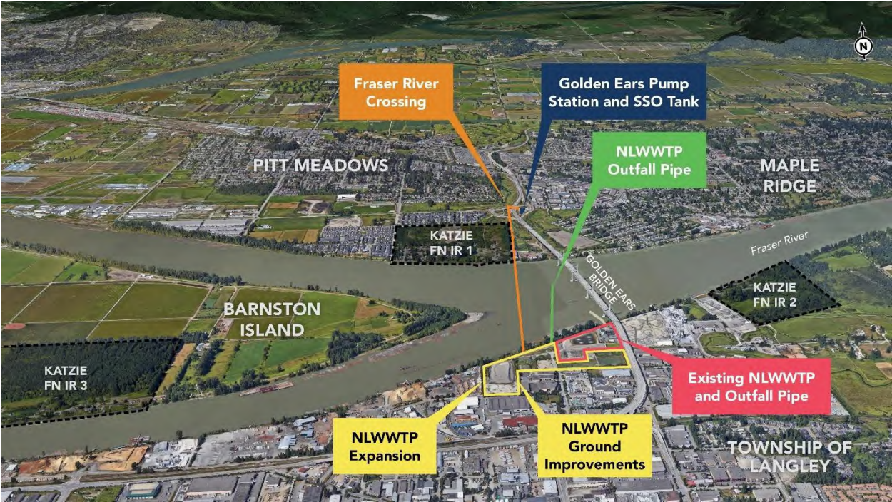
Northwest Langley Wastewater Treatment Plant Program Components
