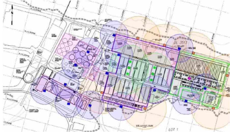
Possible crane locations (24) on a tight site
