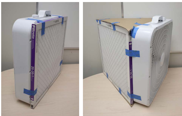
Example of a homemade box fan air filter
